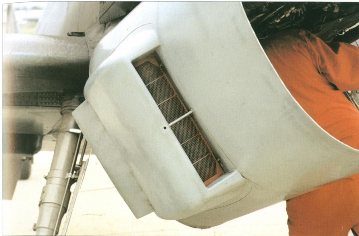
An opened oil cooler cover of Bf 109 G-5. [Paweł Przymusiła]
