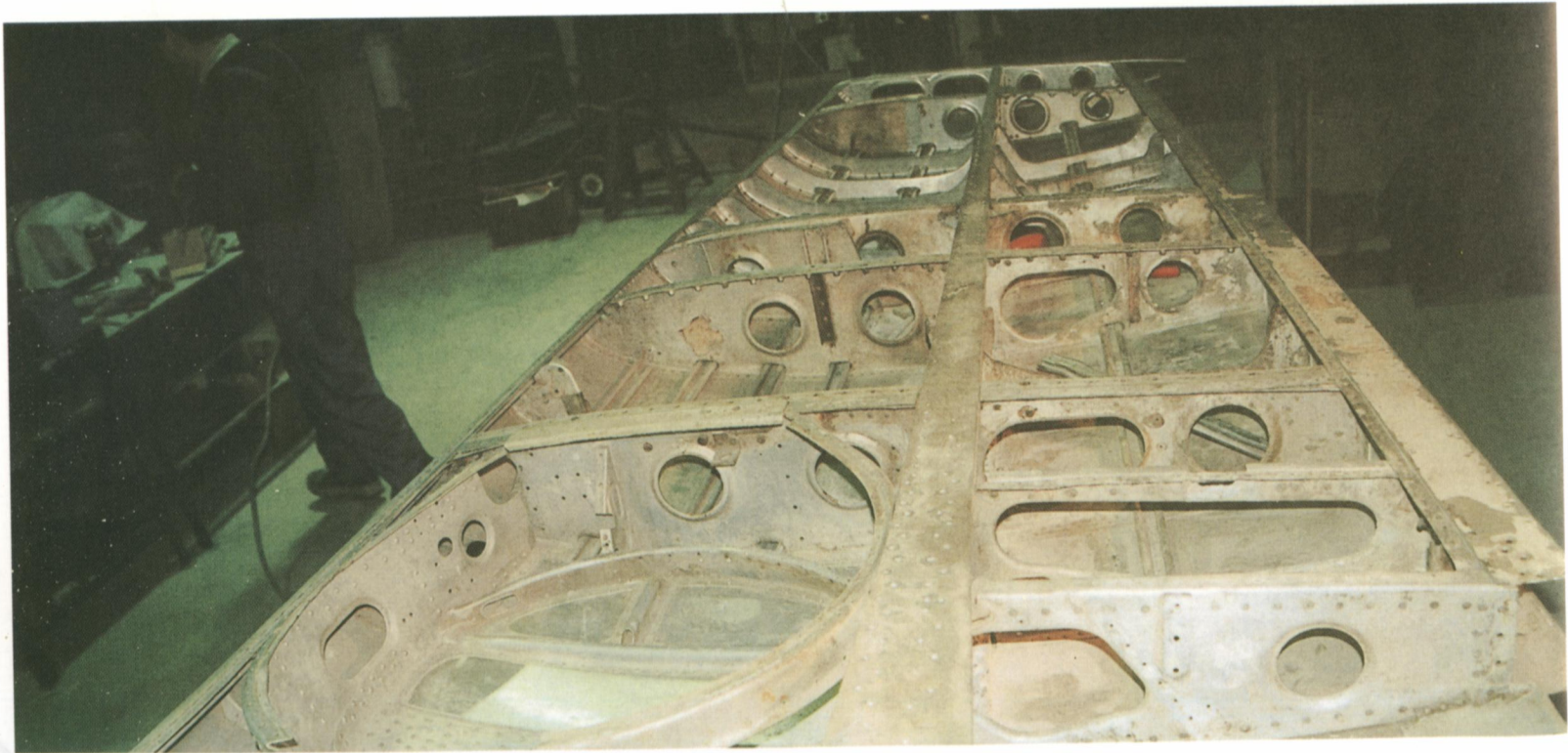
Details of wing construction. [Miłosz Rusiecki]
