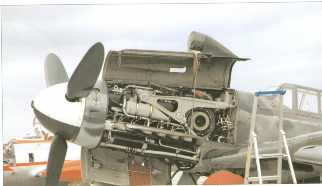
A close-up of engine of Messerschmitt Bf 109 G-5. Note opened engine cowlings. [Paweł Przymusiła]
