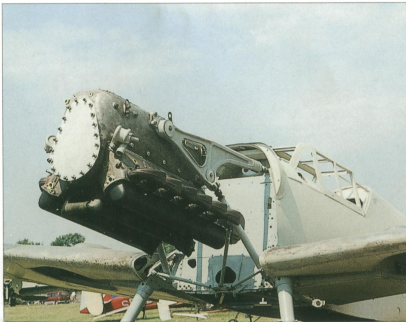
Above. A ventilation cover on DB 605 A-1 engine.[Adam Skupiewski]
