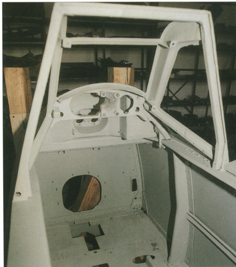
Right. A frame of rear part of pilot's cockpit canopy with baggage compartment. [Adam Skupiewski]
