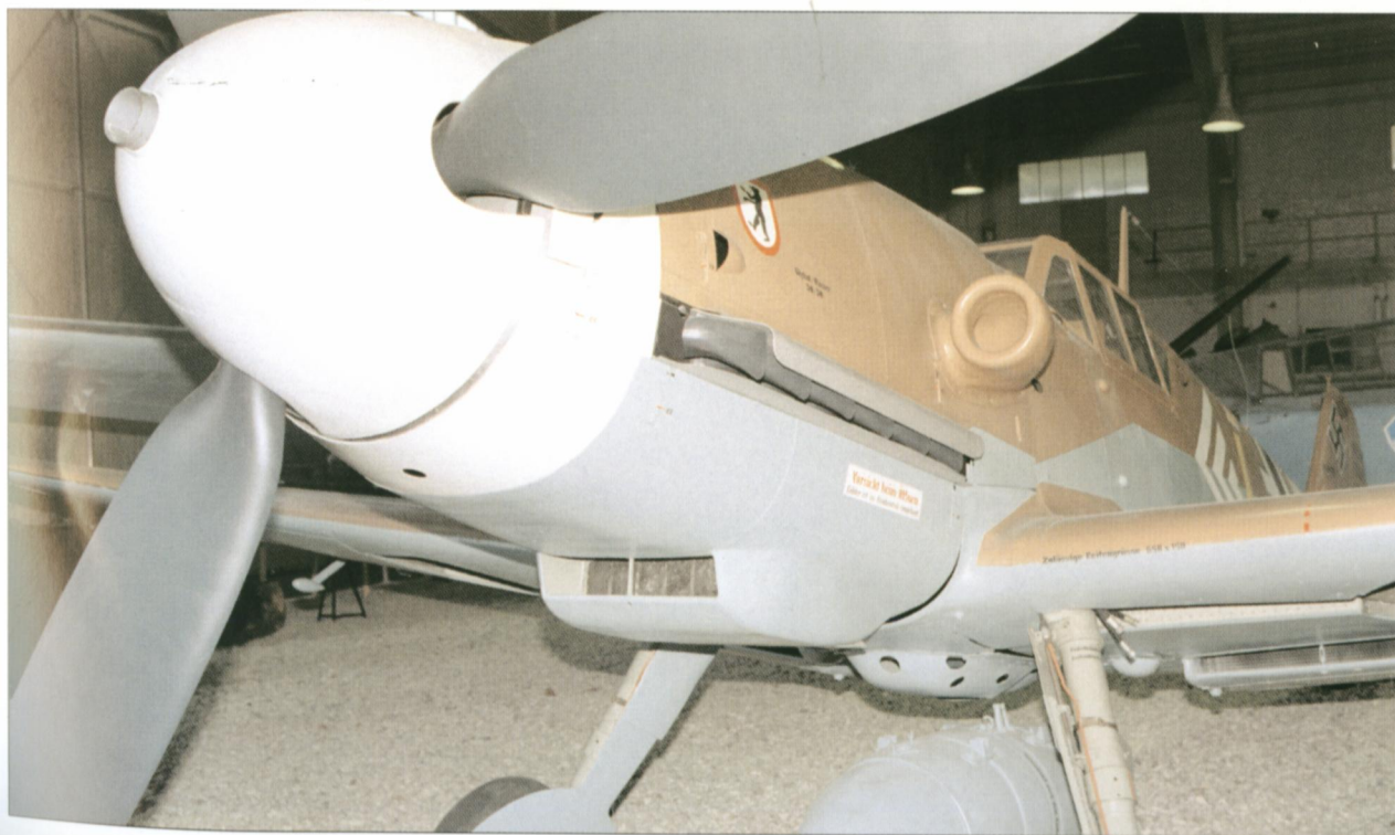
Top. Details of fuselage. Left. Propeller and opened air filter of Bf 109 G-2/R3 Trop. [Paweł Przymusiła]
