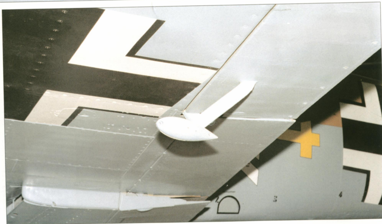
A close-up view of air- leron, flap and aileron balance of Messerschmitt Bf 109 G-2/R3 Trop. [Paweł Przymusiła]
