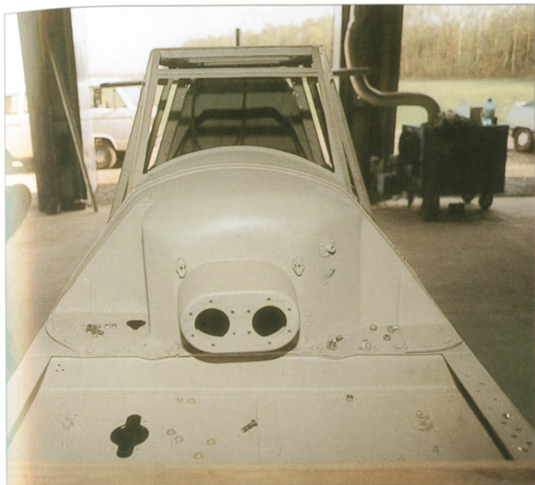
A windscreen frame and the rear part of instrument panel base. [Adam Skupiewski]
