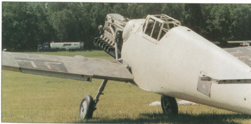
Top. A fuselage of Messerschmitt Bf 109 G-6 Werk Nummer 163306 fitted with tail wheel and main undercarriage. [Miłosz Rusiecki]
