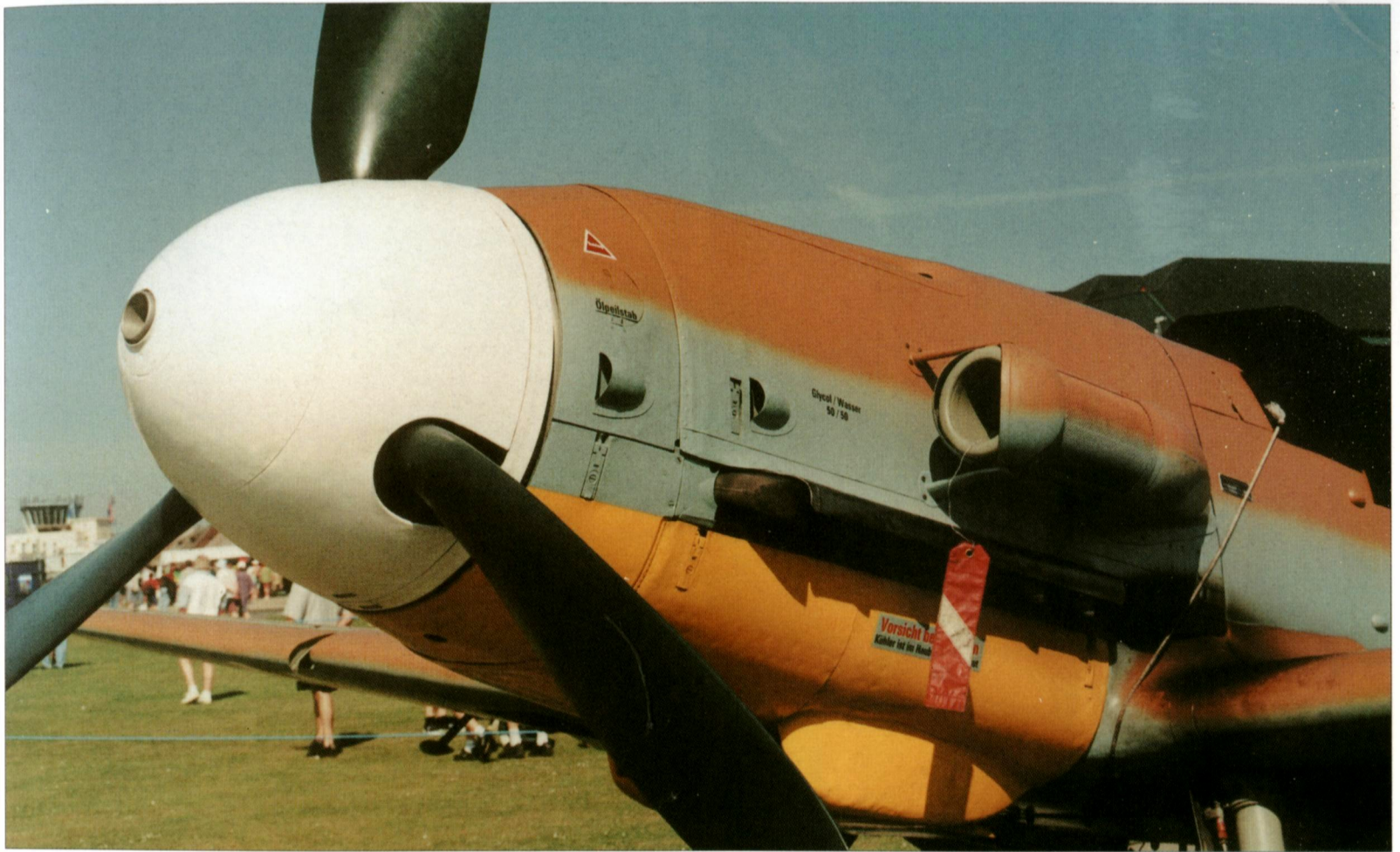
A close-up view of engine, propeller of Messerschmitt Bf 109 G-2 Trop "Black 6". Note opened air filter. [Miłosz Rusiecki]
