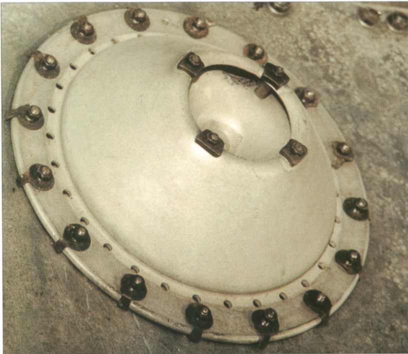
Above. A ventilation cover on DB 605 A-1 engine.[Adam Skupiewski]
