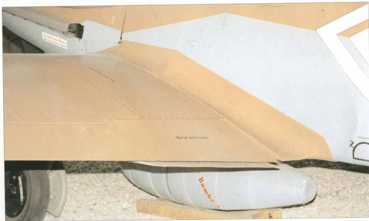
Top. Oil cooler. Right. Wing construction and extra drop tank. [Paweł Przymusiła]
